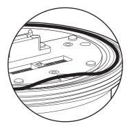
Figure 9. Lightly Lubricate and Install O-Ring
